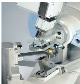
Figure 6: Diffractometer in Transmission Mode
