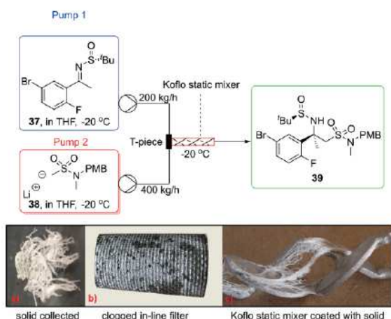
Scheme 12. Reactor fouling attributed to the presence of poly-THF. Reprinted with permission from N. R. Rivera, B. Kassim, P. Grigorov, H. Wang, M. Arme-nante, X. B. A. Lekhal, N. Variankaval Org. Process Res. Dev. 2020 , 24 , 2556–2561. Copyright (2020) American Chemical Society.
