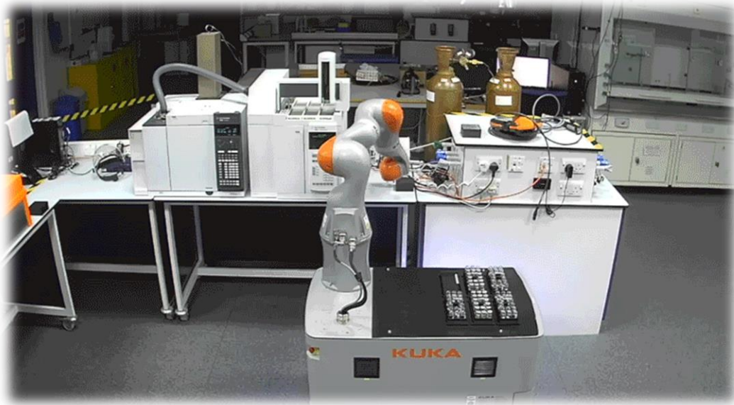
A robot chemist at the University of Liverpool, UK, sifts through thousands of materials to find a photocatalyst. Credit: Univ. Liverpool
